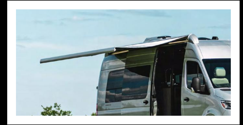
2 The powered awning extends and retracts at the push of a button.
